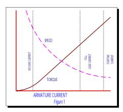
As shown in from the typical performance curves of Figure 1, the high torque at low speed characteristic of the series motor is evident.
