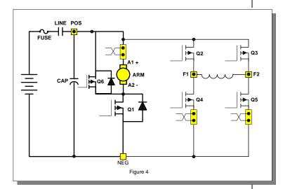
By energizing the transistors in pairs, current can be made to flow in either direction in the field. The field and armature control circuits typically operate at 12KHZ to 15KHZ, a frequency range normally above human hearing. This high frequency coupled with the elimination of directional contactors, provides very quiet vehicle operation.
