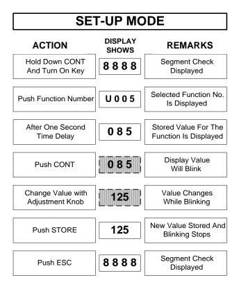
At this point, another function can be monitored/changed by pushing another function number, or the vehicle can be placed in the run mode by holding the **ESC** key down for one second or longer. The display will return to either the diagnostics mode, the BDI display, or a blank display (if BDI is not used and there are no fault codes). The vehicle can now be operated with the Handset connected or the Handset can be disconnected before operation.
