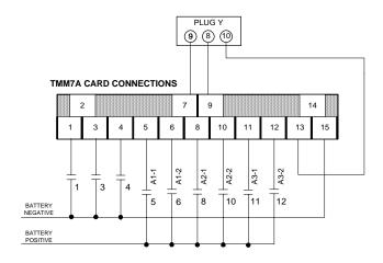
Section 5.4.2 Typical Brush Wear Sensor Connections
